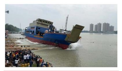
FIGURE 2 SIDE LAUNCH OF MONO HULLED (SINGLE HULL) PASSENGER CUM CARGO FERRY, MV MA LISHA, AT TITAGARH RAIL SYSTEMS LIMITED ON THE BANKS OF HOOGHLY RIVER. THE HEEL (TILT) OF THE SHIP POST LAUNCH IS EXPECTED AND A RIGHTING MOMENT CREATED AS A RESULT OF BUOAYNCY FORCE ACTING UPWARDS BRINGS THE SHIP BACK TO ITS UPRIGHT POSITION IN ORDER TO ATTAIN EQUILIBRIUM.
