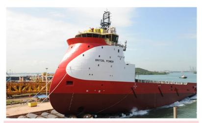
FIGURE 7 LAUNCH OF PLATFORM SUPPLY VESSEL (PSV), BRITOIL POWER, USING AIRBAGS. NOTICE THE INVERTED BOW HULL SHAPE AT THE FRONT. THIS IS CALLED THE 'ULSTEIN X-BOW' DESIGNED AND DEVELOPED BY THE ULSTEIN GROUP. THIS SHAPE AIDS IN REDUCING FUEL CONSUMPTION DUE TO LOWER HYDRODYNAMIC DRAG.
