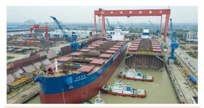
FIGURE 5 DRY DOCK AT COSCO SHIPPING HEAVY INDUSTRIES CO. LTD., YANGZHOU, CHINA. FLODDED DRY DOCK WITH THE SHIP BEING FLOATED OUT OF THE DOCK WITH THE AID OF PUSH & PULL TUG BOATS.
