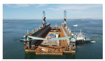
FIGURE 6 JAMAICA'S FIRST FLOATING DOCK, 215 M LONG, OWNED AND OPERATED BY GERMAN SHIP REPAIR JAMAICA LIMITED
