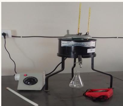
Engler Viscometer test - Rig.
