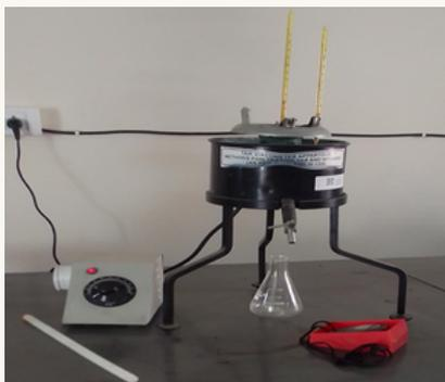
Engler Viscometer test - Rig.
